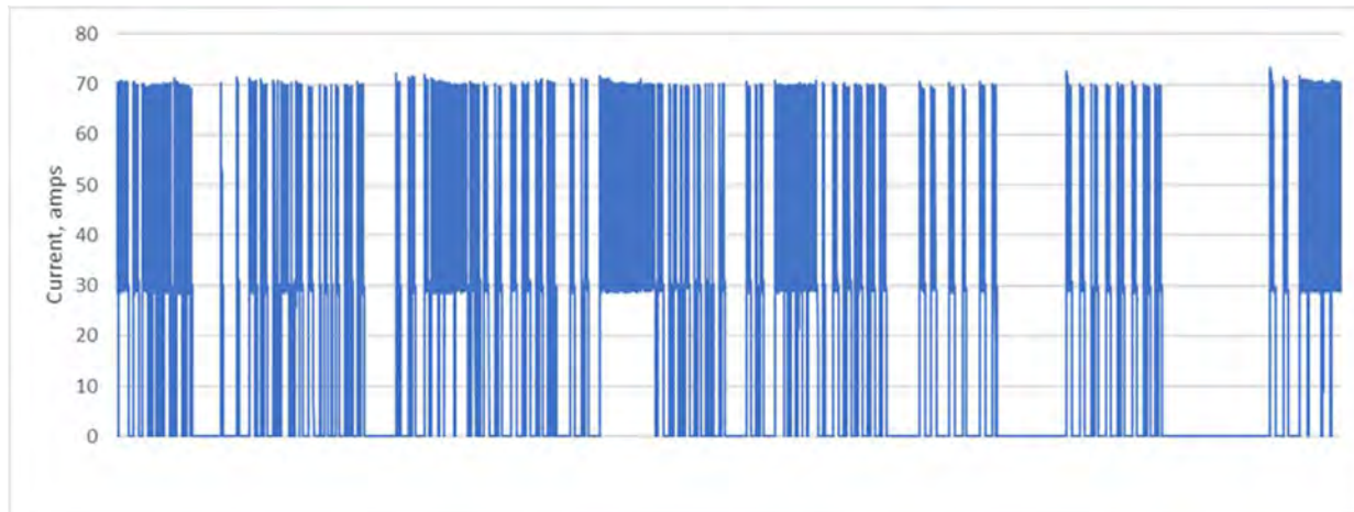
Post Period Compressor Current Metering
